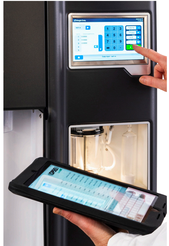
TRANSFER UTILITY ON IPAD TO TRANSFER WEIGHTS TO THE KJELROC ANALYZER
