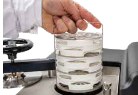
ONE SAMPLE RACK, WITH UP TO 27 SAMPLES, MAKES IT EASY TO ACHIEVE A HIGH THROUGHPUT
